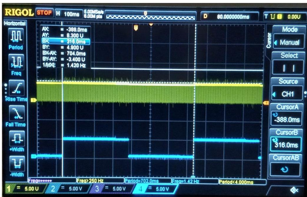
Below, in Figure 11, a comparison between channel three (divide by one-one hundredth) and channel four (divide by one-one thousandth total) is provided.
