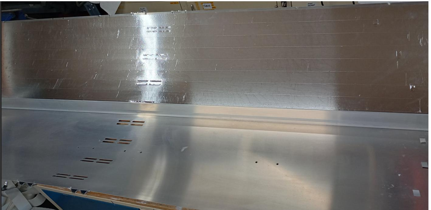
LEDs will be spaced 4" on centers with appropriate focusing lens degree angle. Given large aluminum behaves as a heatsink, LEDs will be super glued directly to aluminum tape. In the event an LED goes bad, or needs replaced, tape should easily peel off and allow replacement.
