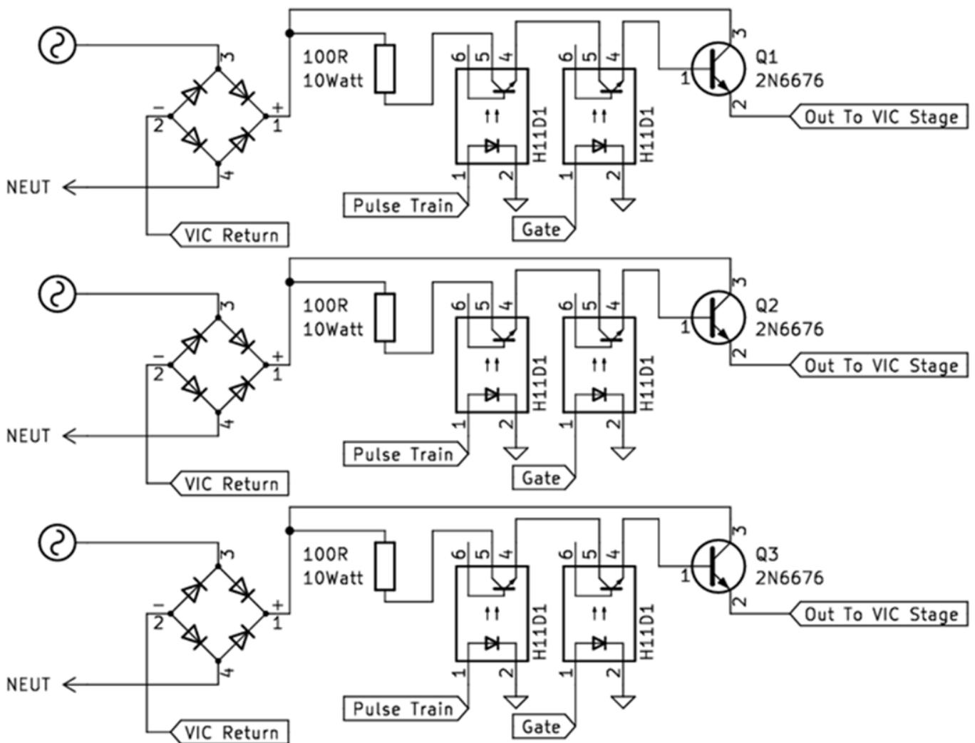
The circuit is composed of three independent power NPN-BJT circuits. The 2N6676 was specified by Stan, however, any of appropriate rating or even modern N-Channel MOSFETs can be used. A rectifier stage produces a variable positive unipolar-pulsating waveform. Each circuit stage has a minimum of two optocouplers that provide electrical isolation between driver and waveform generation means. One provides a frequency pulse train ("Pulse Train"), the second one
