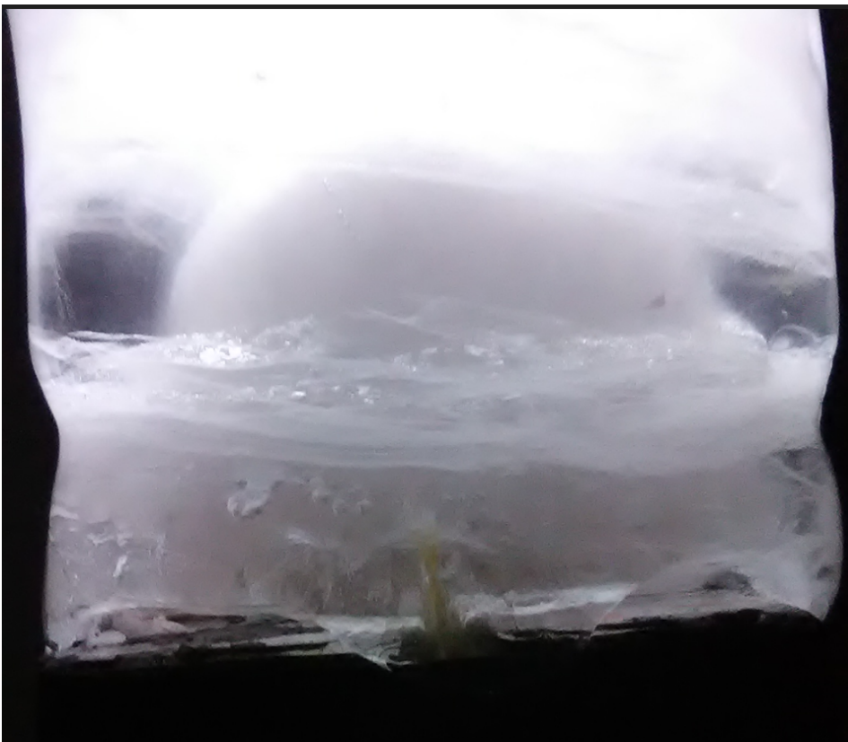
Below photo is of the frozen water out of the cylinder. Illuminating was provided from underneath by pen light. Vortex like geometry can be seen clearly.
