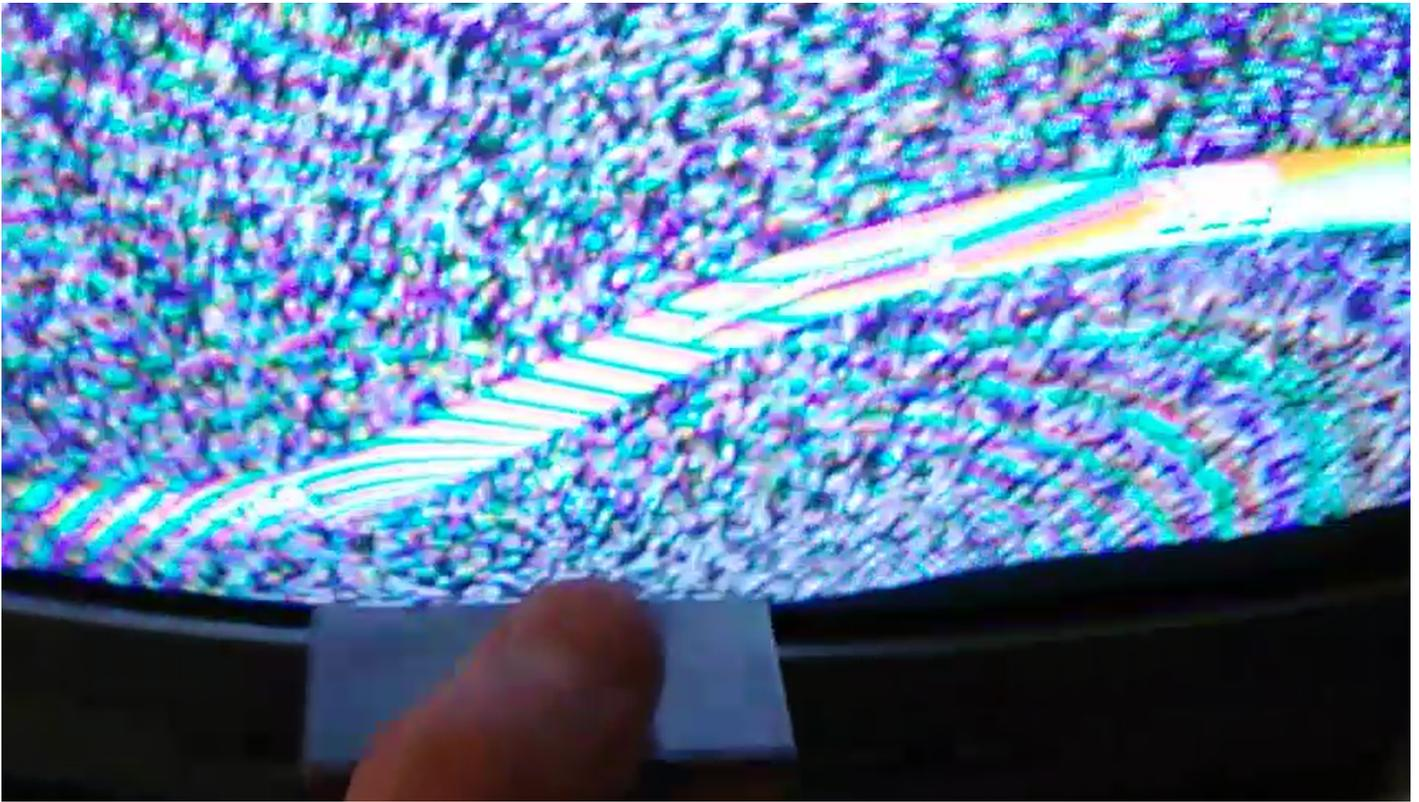
Magnet face being brought close to front of CRT shows the **South pole has a clockwise (CW) spin** direction as shown below.
